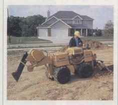
The vibratory plow attachment features a shaker box that delivers 10,000 lbs, of force to the plow for more efficient plowing and increased productivity.
