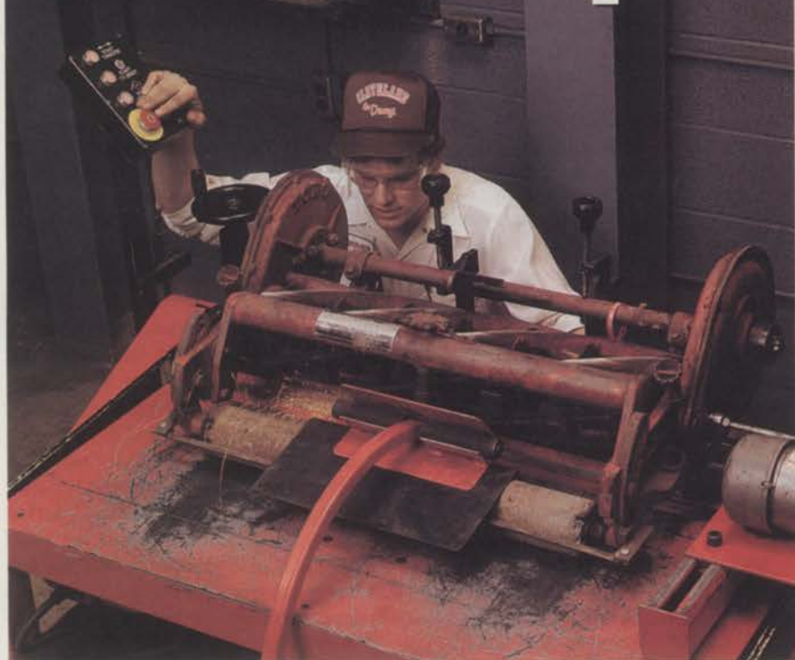
On greens mowers and walkers, the most often used grinding angle is 7° plus a 'dirt factor' of 2°.
