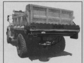
Economical Hiniker tailgate mounted spreaders fit all standard width dump bodies.
