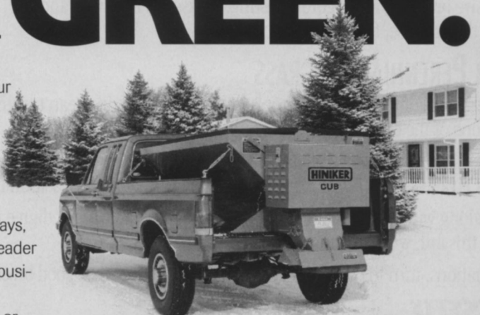
Full-size hopper-type spreaders are available in stainless steel or mild steel versions.
