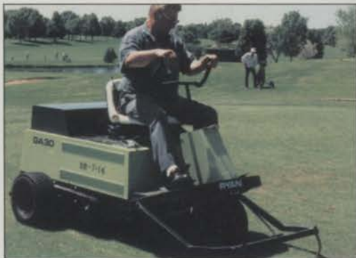
The Ryan GA 30 aerator saves time on tees, traffic areas and approaches. Non-coring tines speed up work in wet weather.
