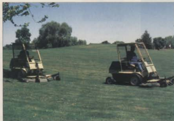
Roughs are mowed with Cushman out-front rotary mowers. They cut faster and better, according to superintendent Arnie Bodhaine.
