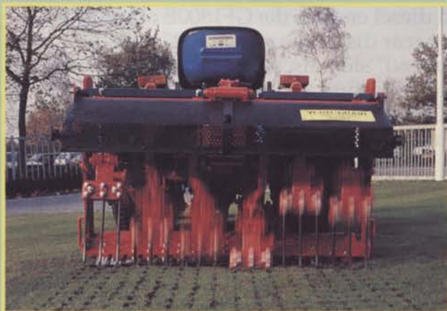
Verti-Drain from Emrex, Inc. aerifies more than 21,000 sq. ft./hr.
