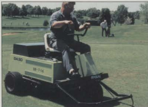
The Ryan GA 30 aerator saves time on tees, traffic areas and approaches. Non-coring tines speed up work in wet weather.
