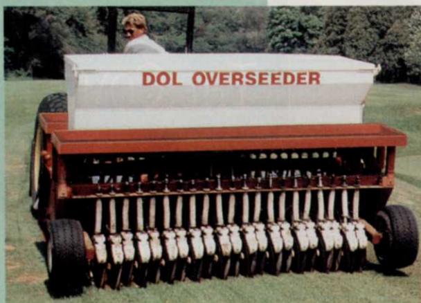
Overseeding, pesticide injection or fertilizing can be done with the Dol overseeder.
