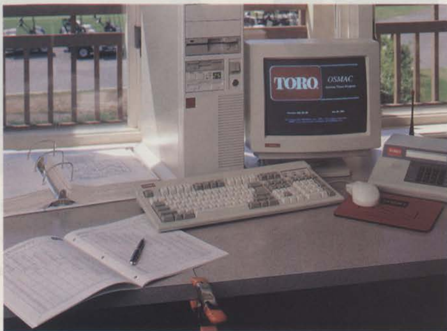
Golf course superintendents continue to replace electro-mechanical irrigation systems with computerized, central control systems. Also, look for more hand-held radios in the coming years.
