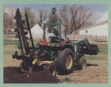
Ditch witch trenchers reach a maximum depth of up to 80 inches.
