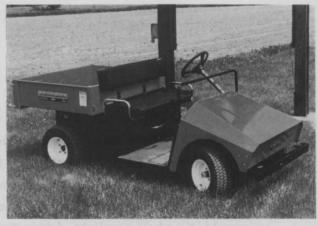
with full differential allows for easy handling in rough terrain.
