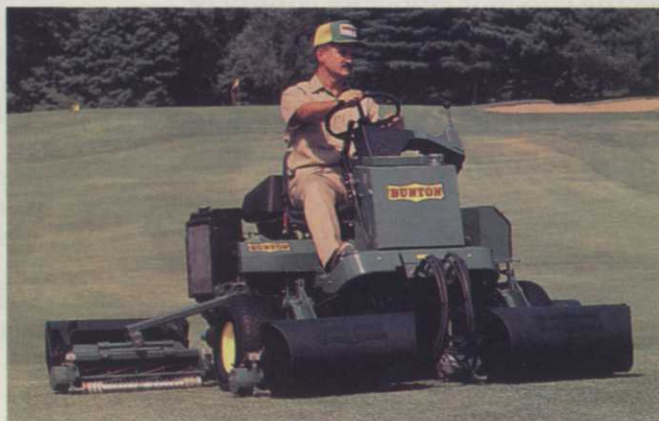
Bunton's fairway mowers have 'cruise control' for steady speed and uniform optimum cutting. (#318)
