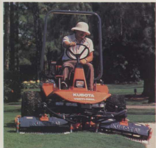
Kubota's Verti-Reel triplex easily converts to a vertical cutter or core buster. (#322)
