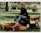
(16.3-HP diesel) or Model I (20-HP gasoline). The deck is specifically designed for mowing rough areas as well as fine turf, using belt driven blades and reinforced deck housing to handle rough conditions. Also new for '94 is a Power Dump Option for the grass catcher. *Circle No.* 146 on Reader Inquiry Card
