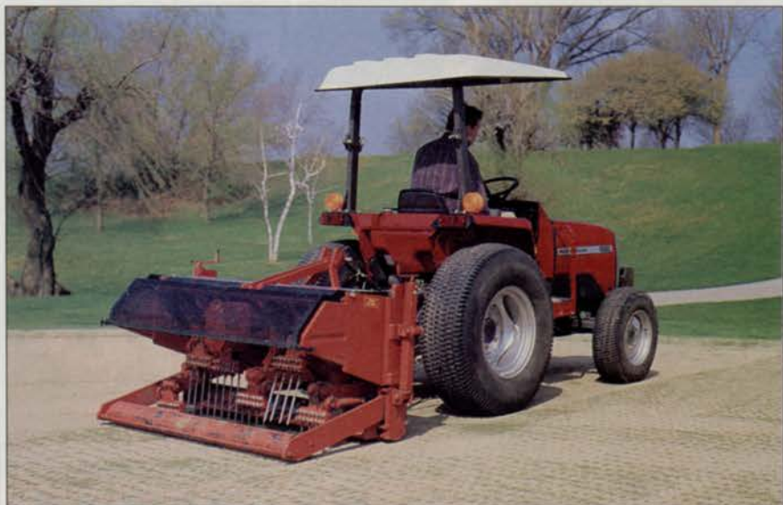
Bryan Wood of Commercial Turf uses a Verti-Drain deep-tine aerator to relieve compaction, increase percolation rates and introduce much-needed oxygen to the soil. The solid tines reach a foot below the surface.
