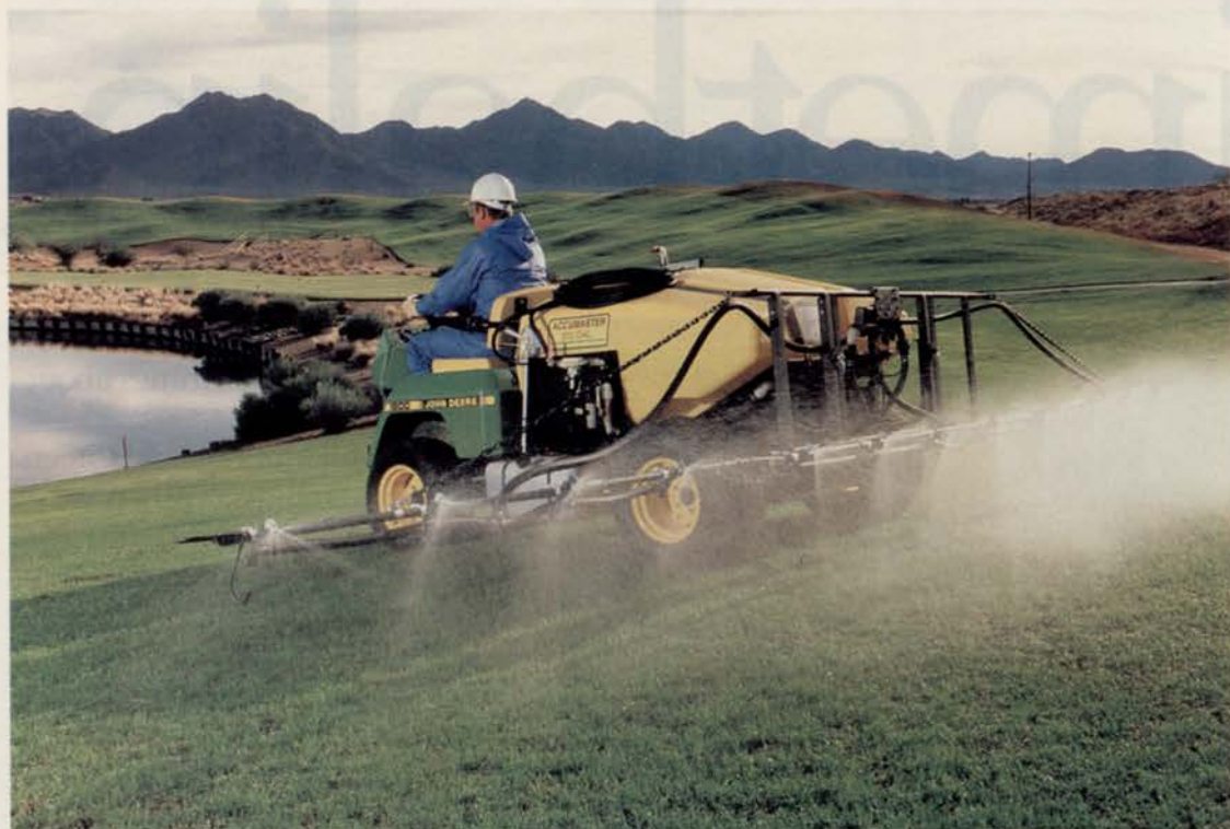
Deere's boom sprayer has a 200-gal. tank and 21-foot chain-supported boom.
