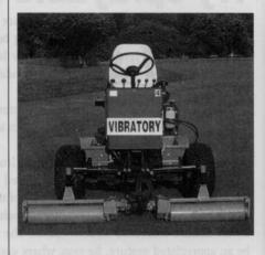
Hydraulic motors provide a source of vibration to create the needed weight to roll a green or tee. According to the company, the reduced weight of this device cuts rolling time in half.
