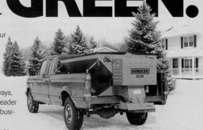
Full-size hopper-type spreaders are available in stainless steel or mild steel versions.
