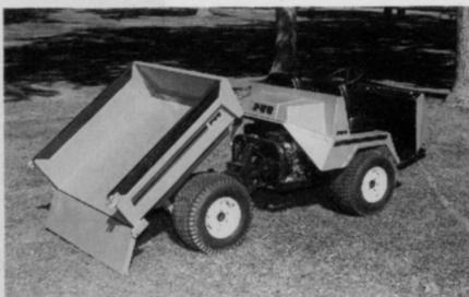
powered by Kohler's V2 20 hp air-cooled industrial engine, is about 10 feet long and weighs 1200 lbs. Pug's towing peak is 3000 pounds. With its four big 26x12x12 traction tires it can go just about anywhere. Its 100 percent automotive drive system has a standard auto clutch, 4-speed synchromesh transaxle, automotive drive line and Spicer differentials that is unique among utility vehicles.
