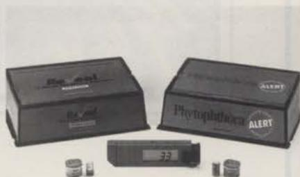
developed to recognize specific plant pathogens. By reading a color change, the user can determine if the pathogen is present and semi-quantitate the pathogen load.
