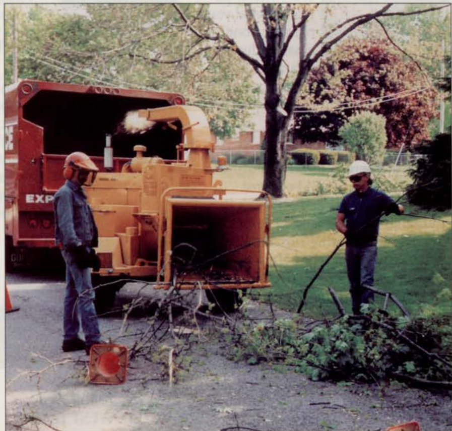
Hard hats, goggles and gloves are required safety gear for chipper/shredder operators.
