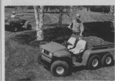
The 10-hp Gator 4 x 2 has on four wheels, with 2-wheel drive and differential lock. A single-cylinder, air-cooled engine supplies the power. The cargo box is 10 cu. ft., and hauls up to 500 lbs.
