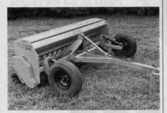
The seed box is a welded, water-tight compartment with a double-wall lid and a V-shaped bottom for complete clean-out of seed. Its fluted seed cups meter precise amounts and can be set to accommodate a wide range of seeding requirements.
