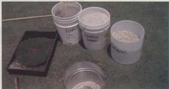
Stainless steel containers filled with the same layers of materials as the green allow researchers to capture and measure leachate.
