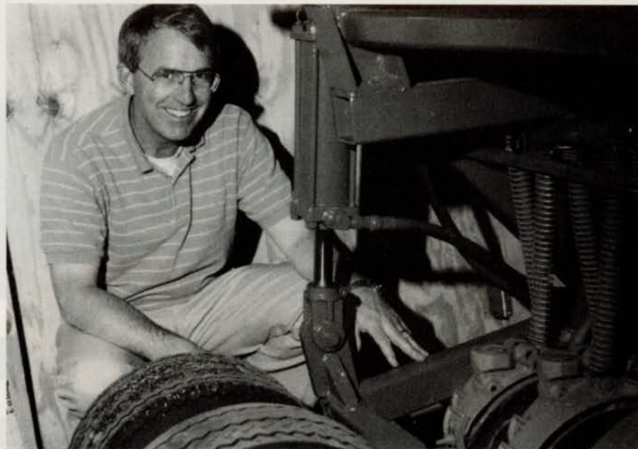
Bob Wicker says the colter/spring arrangement won't damage sprinkler heads during application.
