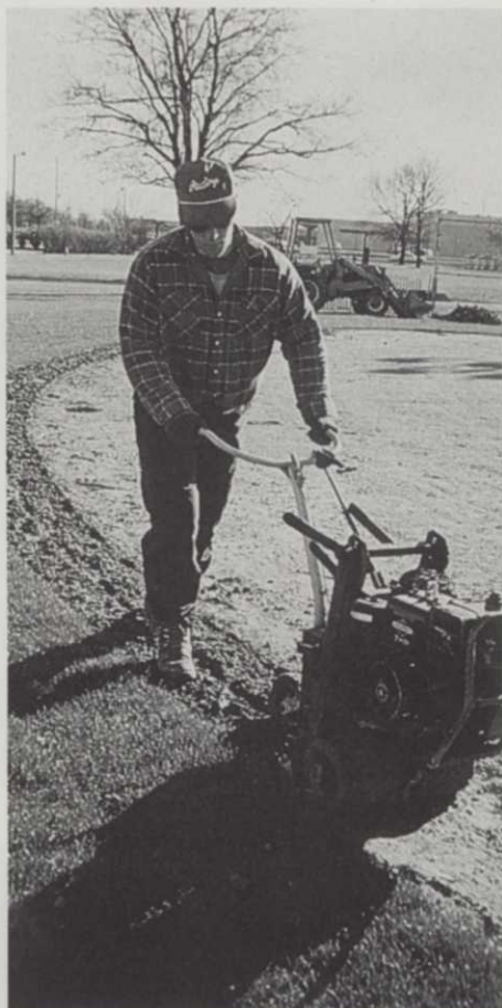
Al Liebert cuts sod during field renovation along the arc edge.
