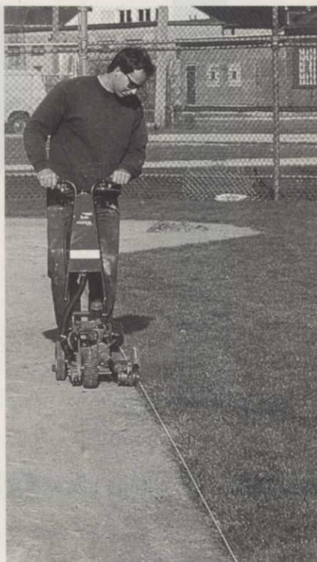
Mike Brouillard uses a sidewalk edger to trim about two inches of infield turf.
