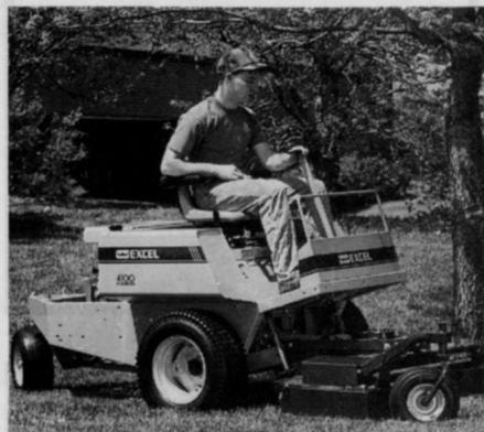
drive wheel motors. According to Excel, the drive concept eliminates the need for high maintenance chains, sprockets and transaxles.
