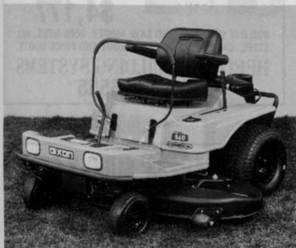
The mower's drive system uses twin hydrostatic units with hydro gear drive. It features a large capacity reservoir, separate fans, and a charge pump to actively cool the hydraulic fluid, a feature important for commercial users.
