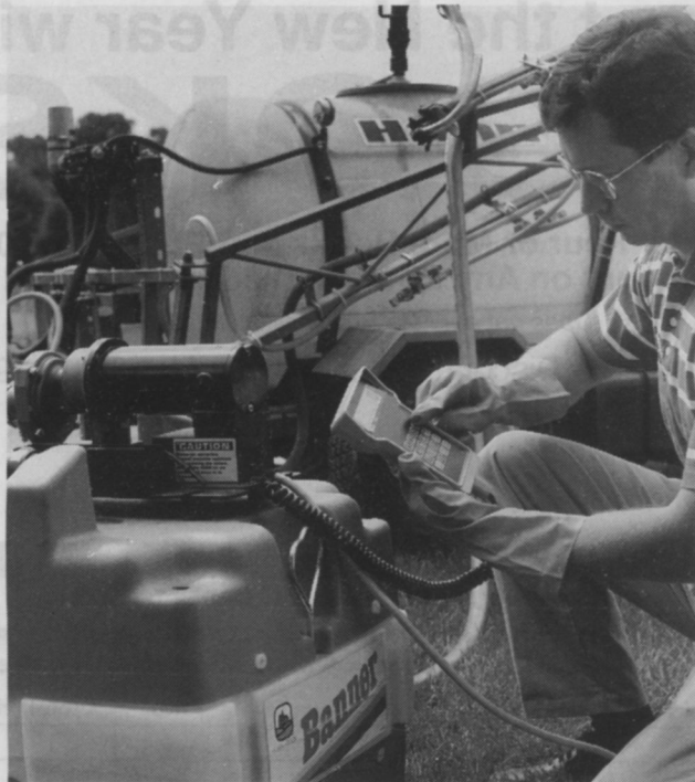
Turfpak features a 15-gallon returnable container, electronic control module and dry-break couplings.
