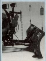
Western Products' UniMount System allows quick and easy removal of a Western Snowplow from the front of a truck. Four pins and two electrical plugs are all that's needed to attach or remove the UniMount System. Western's hopper-type sand and salt spreader is a self-contained material spreader for ice control on driveways, roads, parking lots and sidewalks. Mounts easily on pickup, dump or platform trucks.
