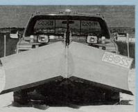
straight blades and blades that are hinged in the middle so they can be used as Vblades to cut through drifts or inverted Vblades to carry snow across a parking lot. The Boss also overs Rapid-Tach, the truck-to-plow quick hitch, and several dif-
