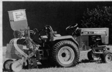
Tractors are easily modified to perform polymer injections.
