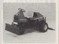
rake for smoothing, a mid-mount cultivator to lift and loosen, and a front blade to push sand or other soil types. Accessories are operated from driver's seat.
