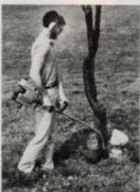
**3) Balance and maneuverability?** On some models, the engine is placed at the back end of the unit; on others, it is down at the head. In either case, balance is the key to efficient user operation.
