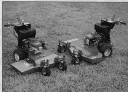
provide better air flow. In addition to side discharge, the mower also offers the option to mulch or bag clippings.
