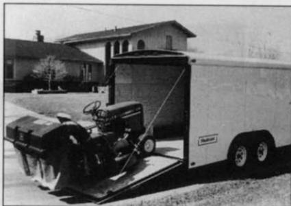
and 8-1/2 feet are available in lengths of up to 37 feet. Fifth wheel and gooseneck models are available up to 48 feet long in widths of 7 and 8 feet.
