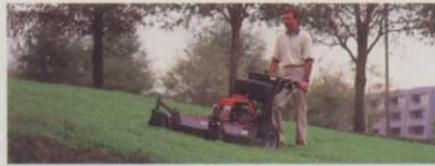
that powerful Honda 13 horsepower OHV engine. Plus, those slopes aren't tiring you out. That's because the twin hydraulic pump system lets you control power to each drive wheel independently. You simply balance the power with two levers and the mower tracks straight, even on slopes. You do more work with less fatigue.
