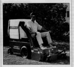
With the Lynx 2000, the operator has the versatility of collecting clippings or, by changing a pin and removing a quickchange panel, clippings can be discharged back to the turf.
