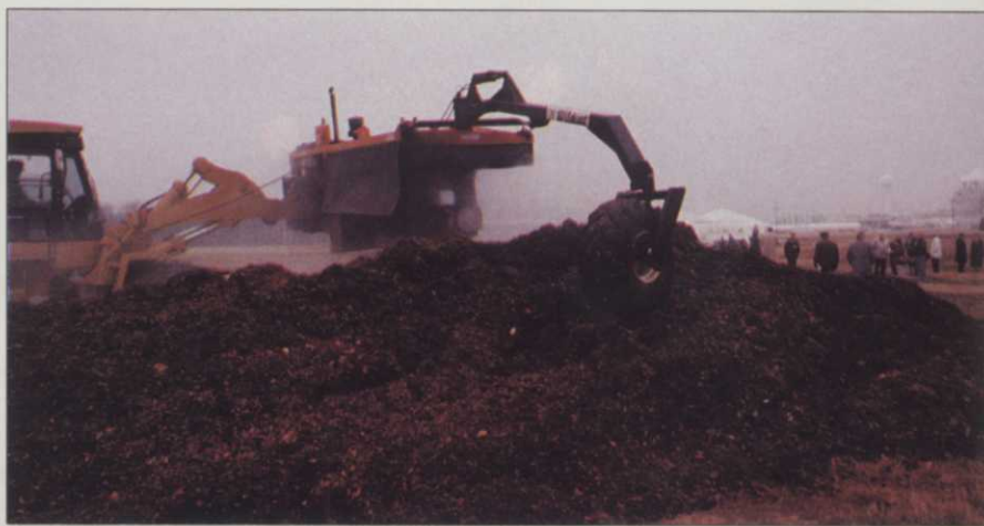
The Wildcat Turner allows air to circulate through developing compost at the Scotts/Hypoxex site in central Ohio.
