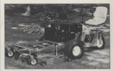
company's exclusive Trans-Guard system. According to Exmark, Trans-Guard reduces peak loads by 30 percent, which extends transmission life and helps avoid costly engine repairs.
