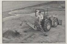
implements designed for the versatile Band L-Series tractors. It digs to a depth of 7.5 feet and has a force of 2950 pounds.
