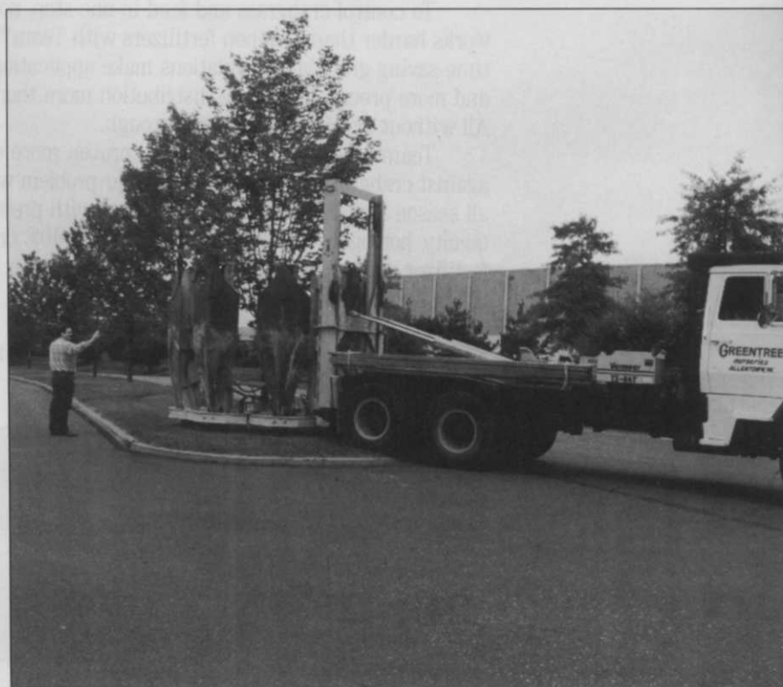
Vermeer TS 84T prepares to place the tree in freshly-dug hole at office complex.
