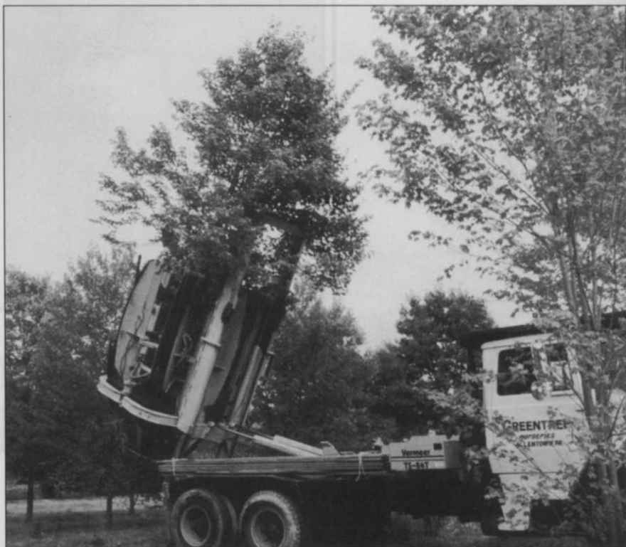
Vermeer TS 84T tree spade removes a tree from the Greentree farm.
