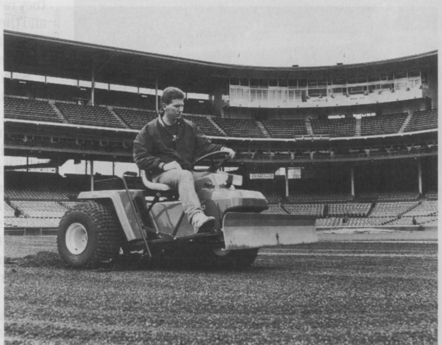
Deere's 1200 bunker and field rake breaks up infield soil at Wrigley Field in Chicago. A center-mounted scarifier and rear-mounted field finisher perform the task. A front-mounted blade helps to move the material.
