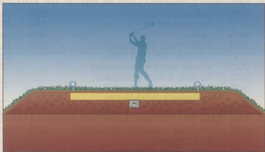
Sand below the playing surface eliminates compaction, provides adequate tee drainage. Thicker soil on the slopes directs moisture towards the drain tile. Better drainage means easier mowing.
