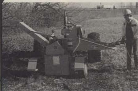
PTO Powered featuring 7" diameter capacity, spring loaded throwout clutch and a 500 lb. cutter drum. Reduces brush & limbs to a mulch chip.
