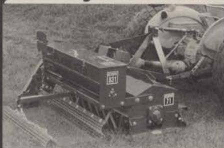
Plant water-absorbing polymer to reduce amount and frequency of watering. 48" swath with blades on 6" centers.
