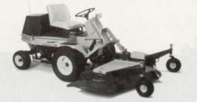
ANSWER: The Cushman 809. This new gasoline water-cooled Front Line® Mower features a 27 hp., 3-cylinder Teledyne-Wisconsin engine that cuts through the toughest, tallest grasses with power to spare. It's quiet and it stays cool for years of top-cutting performance. For all the facts, return the reader service card in this publication today.
