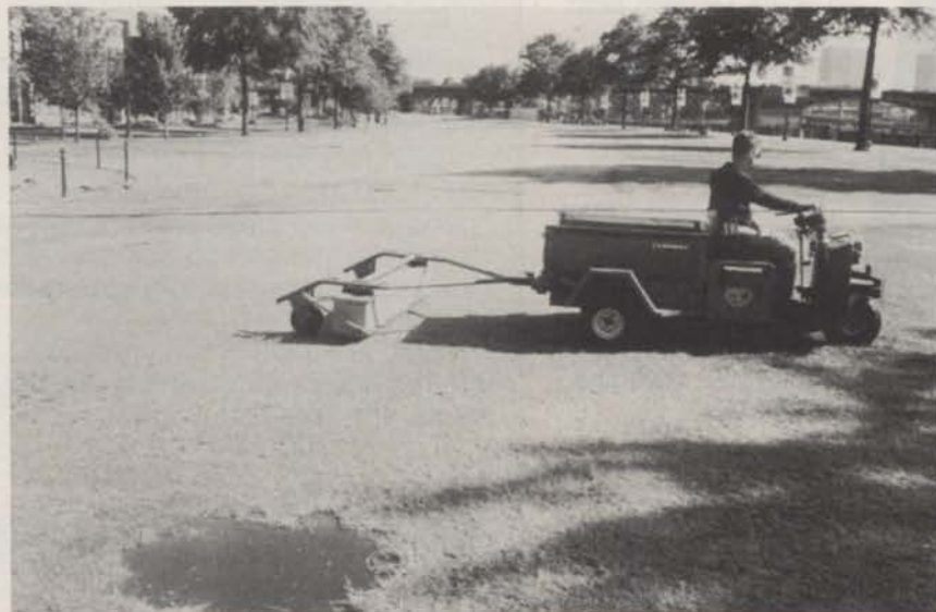
Following a major festival in mid-June, the maintenance crew drags a magnet over the turf to remove bolts, nails, bottle caps, wire and other metal.
