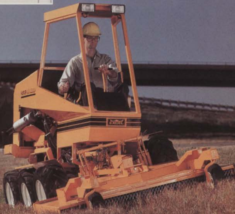
Diesel-powered Hustler 640 Hillsider with the 72" Heavy-Duty Dual-Trim mower deck.
