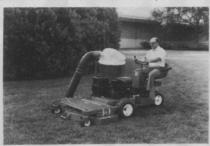
and gauges on the instrument panel. A softer seat, hydraulic deck lift, 60-inch mower deck and tool/debris box are all standard. A 5.6 bushel Grasscatcher attachment is available. Circle No. 198 on Reader Inquiry Card
