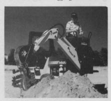
ground boring as well as removing rocks, or digging to gas or water mains. It uses two control levers, one for boom and swing, the other for dipperstick and bucket operation. A third lever controls the 69-inch wide backfill blade, which acts as a stabilizer. The operator is situated high for ex-
