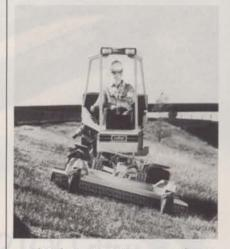
This design is unique, according to Excel, because the engine is also held level, allowing for proper lubrication at all times. The tractor's weight distribution remains constant over the drive wheels for unmatched traction and balance.
