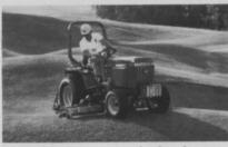
tractor's open center hydraulic system. As a safety measure, reels stop when lifted out of working position.
