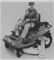
a true zero radius turn and simple hand lever controls that eliminate all footwork.
