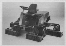
back suspension seat with arm rests, and four-inch fore and aft adjustment; power steering and tilt steering wheel, readable gauges and well-positioned controls; and all-hydraulic design for raising and lowering cutting units.
