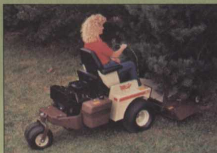
Outfront deck design lets you reach hard-to-mow areas that belly-mount mowers can't get to.
