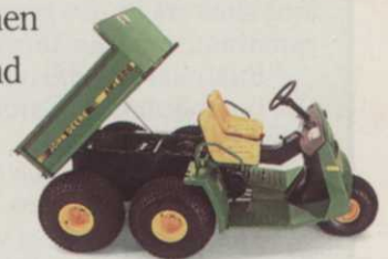
Hydraulic dump option on the AMT 626 allows you to empty its cargo box from your seat.
