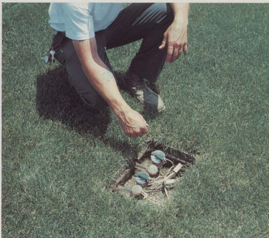
Tensiometers can determine the point at which soil saturation, field capacity and permanent wilting occurs within a particular soil profile.
