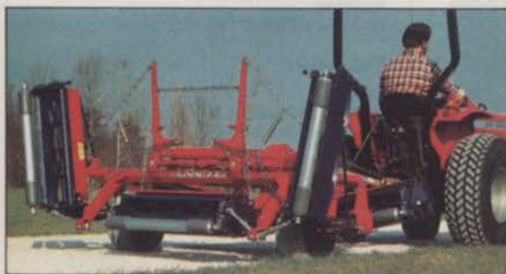
2. Hydraulic lift for easy transport or storage
