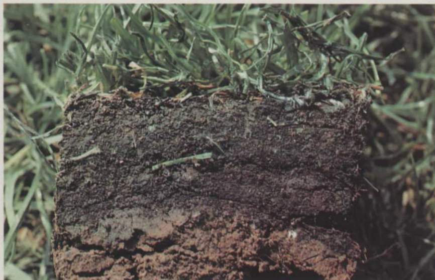
The deep penetration of blue dye into this turf following application by the RainSaver Jr. shows the advantage of subsurface injection.
