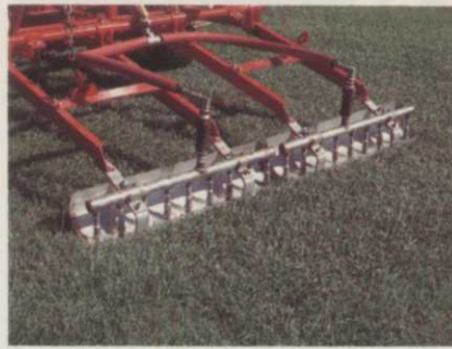
Cross Equipment's Injektaspray system has a low-height, low-pressure topical spray followed by a high-pressure ground surface injection.
