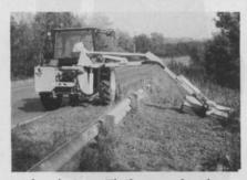
ter head sizes. Flail cutter heads are available in 40-, 48-, and 60-inch cutting widths. With the cutter head fitting, the P12 offers a horizontal reach of 144 inches. The P15's reach extends to 187 inches.
