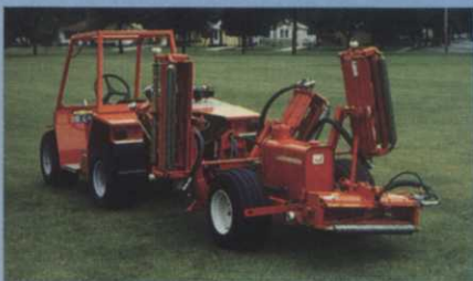
A powerful 5-Gang Hydraulic Ranger with a 133" cutting swath is also available.
