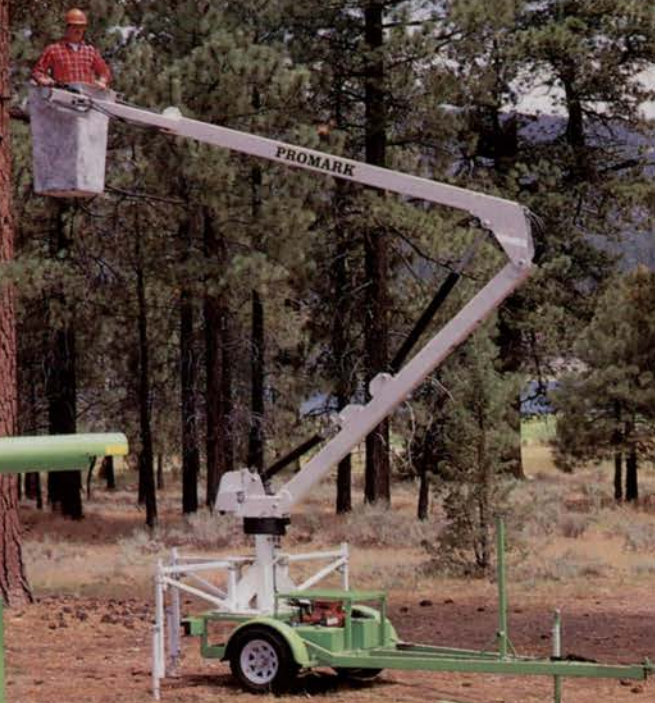
Model PAL Aerial Lift/Trailer (top)
